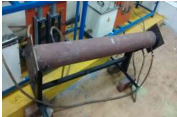
Fig. 4 Fabricated setup of shell and tube heat exchanger
